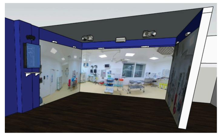
**Please note** that each projector has a maximum display width of 4 meters, please use this as a multiple factor when calculating your image space, there are no multiple maximums. It is good practise when designing a 270 degree experience to allow for a break out zone at the front of the projection space.
